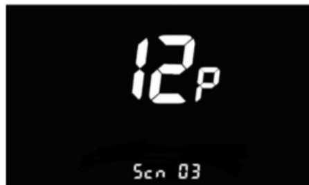
Figure 6-12 Pedal assist strength setting interface
