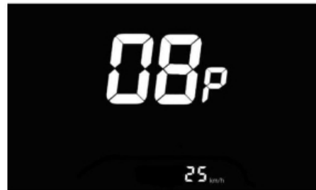
Figure 6-8 Speed limit setting Interface
