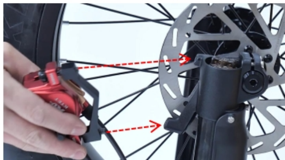
03 Align the screw with the hole
