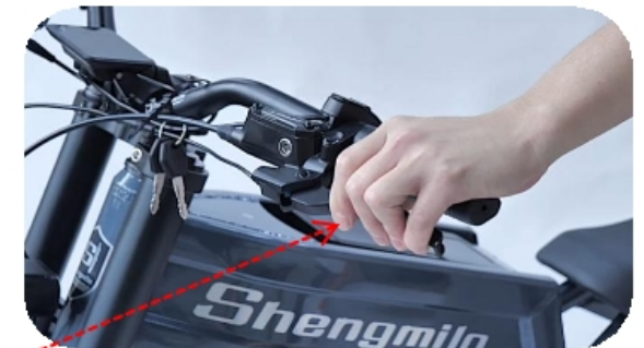
05 While tightening the screws, check the brake performance
