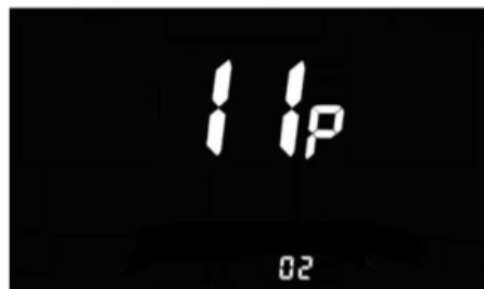
Figure 6-11 Pedal assist sensitivity setting interface
