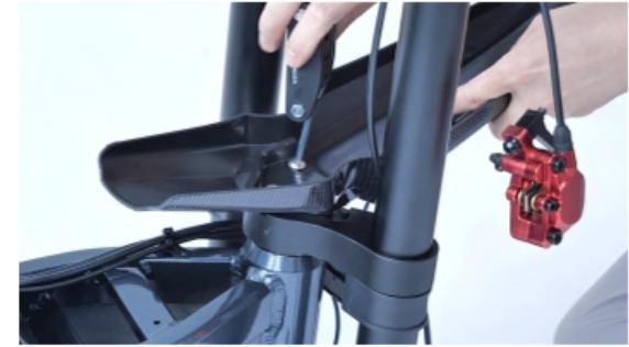
03 Align the screws with the holes and tighten them with tools.
