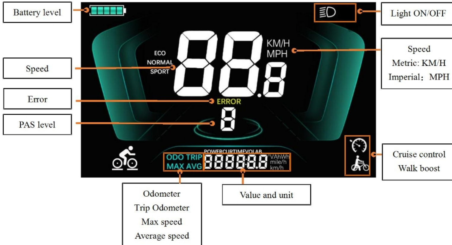
Figure 4-1 YL81F-H functional area distribution interface
