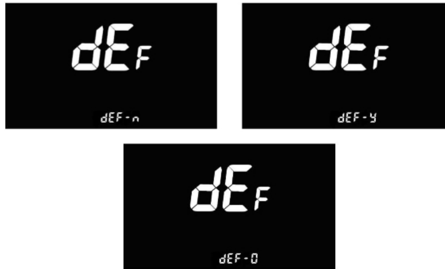
Figure 7-1 Restore factory default parameter setting interface
