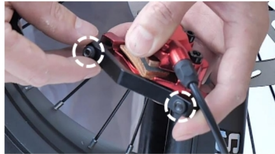
02 Remove the screw washer as well.
