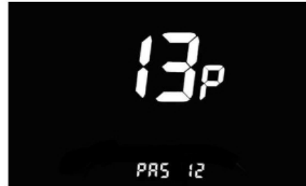
Figure 6-13 Number of pedal assist sensor magnets setting interface
