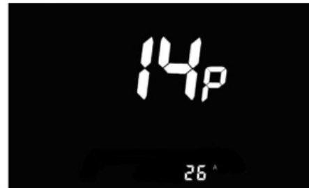
Figure 6-14 Controller current limit setting interface
