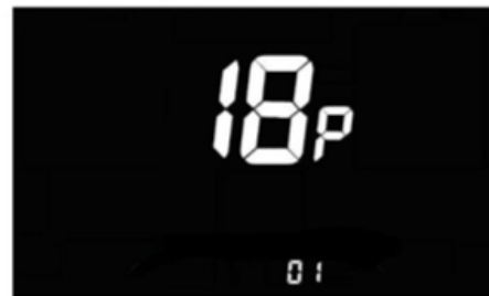
Figure 6-18 6km/h walk boost setting interface
