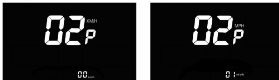
Figure 6-2 Metric and Imperial setting interface
