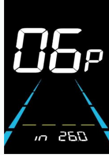
(06P is shown in the picture) Wheel diameter setting interface
