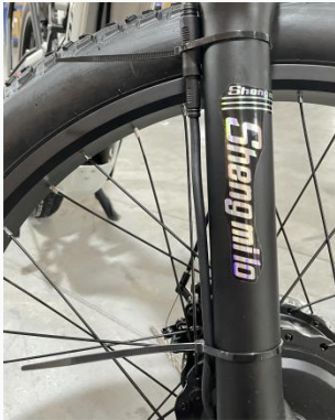
(1) Secure the wire to the fork with zip ties.
